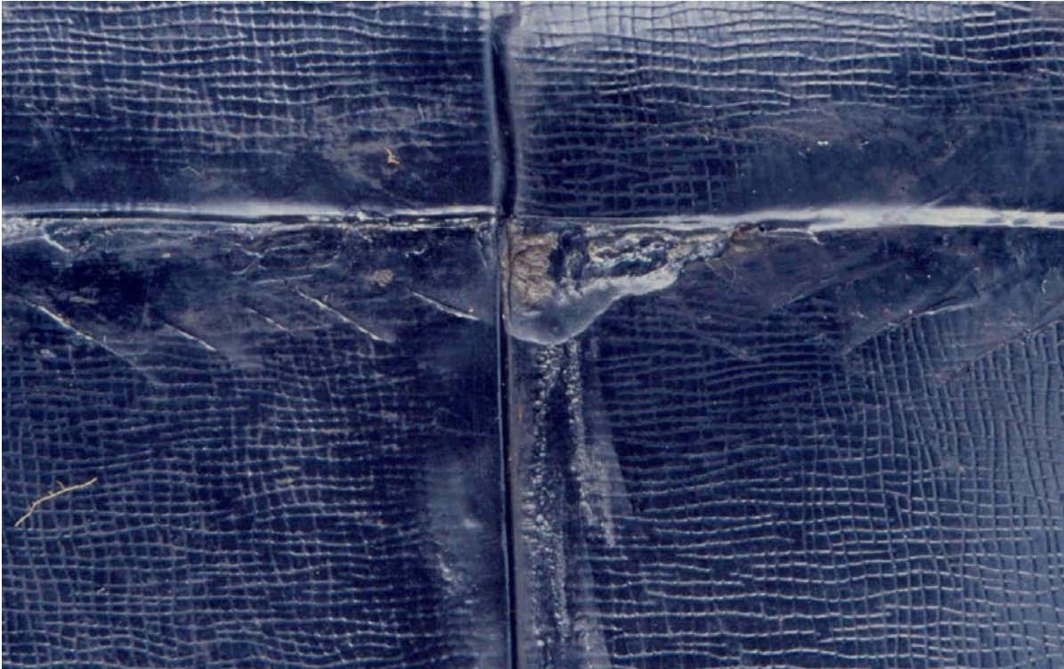
Figure 3: Sheet surface (T joint)
