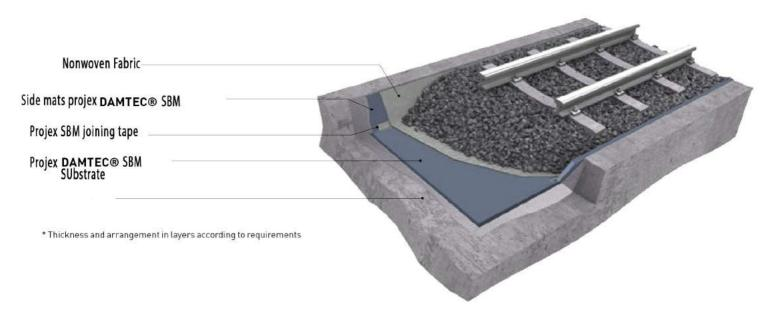
Embedding the entire track system intDAMTEC® products creates a mass-spring system that with the appropriate dimensions acts as highly effective acoustic and vibration isolation. This effect also occurs with complicated track geometries. In mass-spring systems, DAMTEC® products are installed at points, in strips or covering the whole area. The mass-spring systems in the form of track supporting layers and track troughs are generally individual solutions that we are happy to work out for you.
