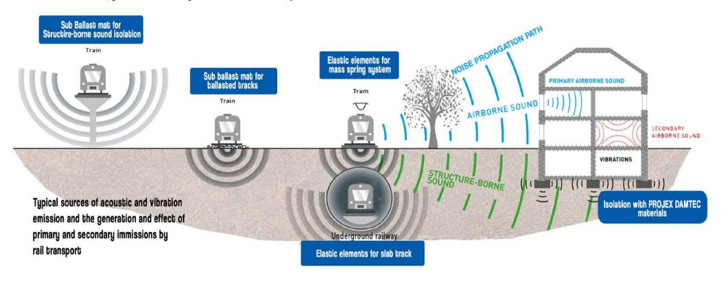
These vibrations are transmitted to the substrate via the track system and propagate from there as structure-borne sound. If buildings are located adjacent or in close proximity to the track system, then a transfer takes place through their foundations. The buildings begin to vibrate, and if this becomes intense enough, it is also interpereted as a noticeable vibration or disturbing noise.
